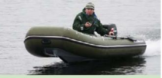
Test results conducted on March 2010 by Boats and Yachts Magazine with different payload. Conditions: Air temperature – 26 Fahrenheit (-2 C) Water temperature – 38 Fahrenheit (4 C) Wind – 2 knots (1-2 m/c) Wave height – 0-4 inches (0.0-0.1 m) Outboard motor – Suzuki 15
